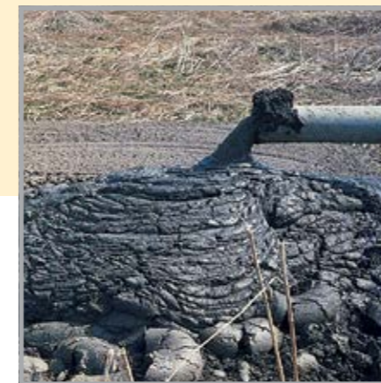
River sludge with high dry solids content has short drying times
