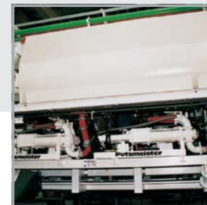
Left: A KOS 1050 pumps the injection mortar behind the ring segment Right: Space-saving installation with two KOV 550 Duo underneath a 6 m 3 agitating trough
