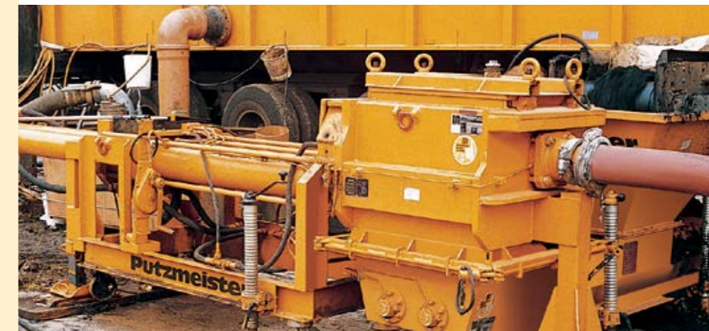
Mobile dewatering and pumping station
