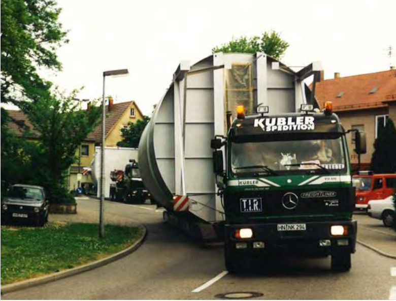
Fig. 106: Transport of the complete manu- factured silo with 5.5 m diameter and 13 m total length to the installation site
