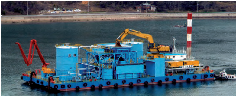
Fig. 71: Floating processing plant with placing boom, excavator and various structures
