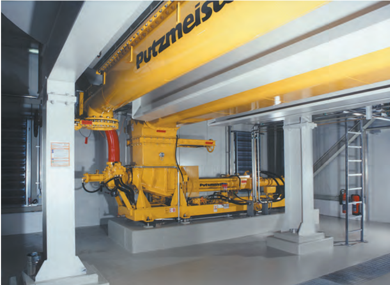
Fig. 120: Silo discharge screw feed the solid pump
