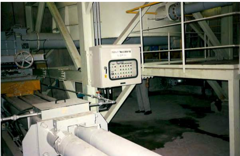
Fig. 102: The construction height can be minimized with the double combing pre-pressing screw
