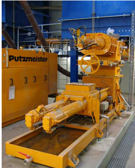
Fig. 113: Discharge of receiving bunker on level minus 6.5 m auger feeder, flat gate, piston pump with oil pan
