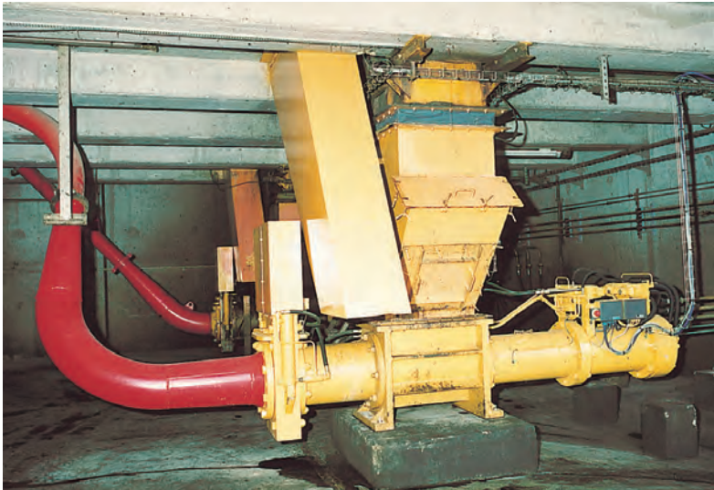
Fig. 50: Single piston pump with gate valve
