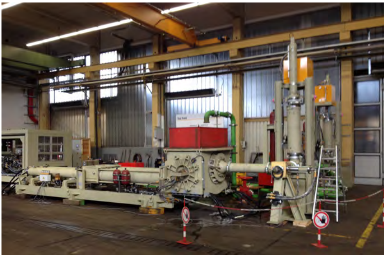
Fig. 137: KOS with HPD pulsation dampening system on the Putzmeister test field
