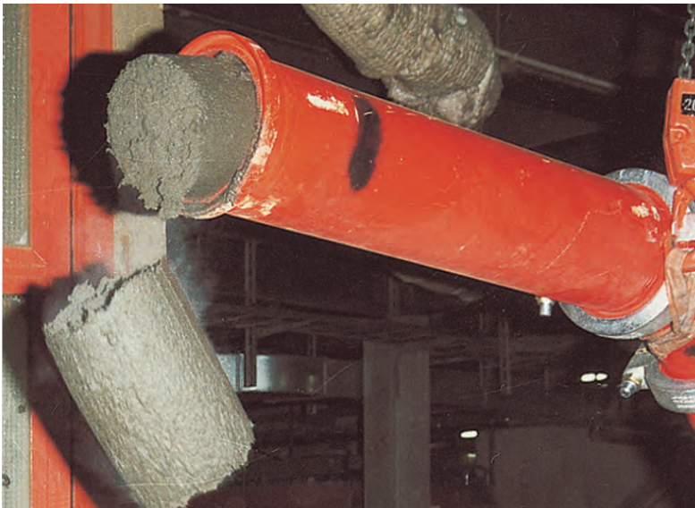
Fig. 3: A high grade of dewatered sewage sludge with 47% solid content
