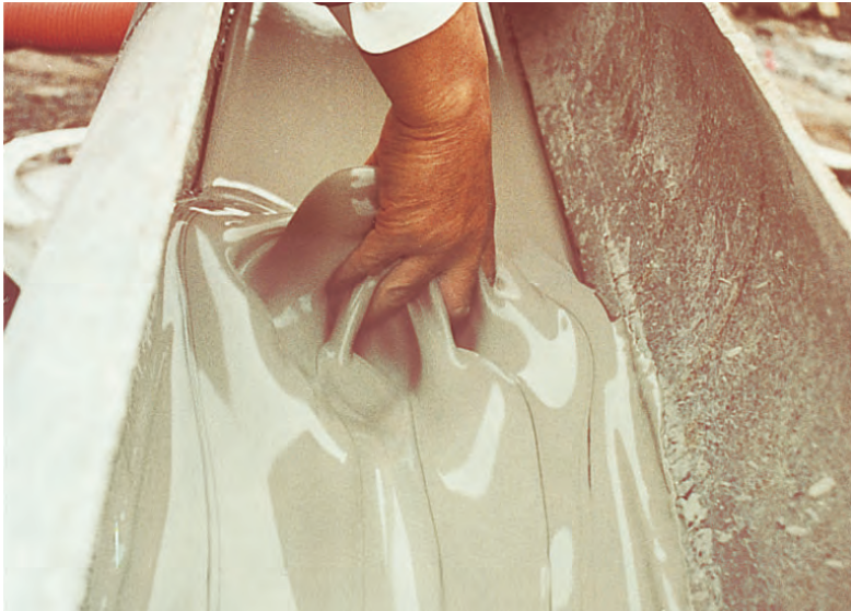
Fig. 43: A suspension of fly ash and water is especially abrasive and extremely thixotropic. Solids content 65%
