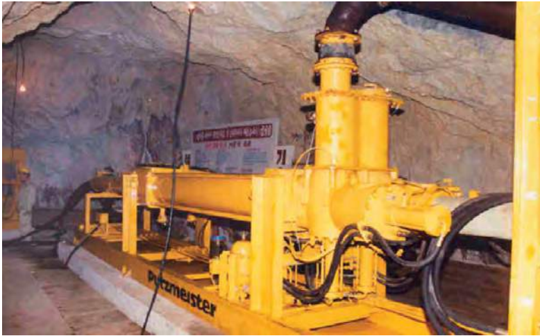
Fig. 60: Seat valve pump with mounted damping vessel
