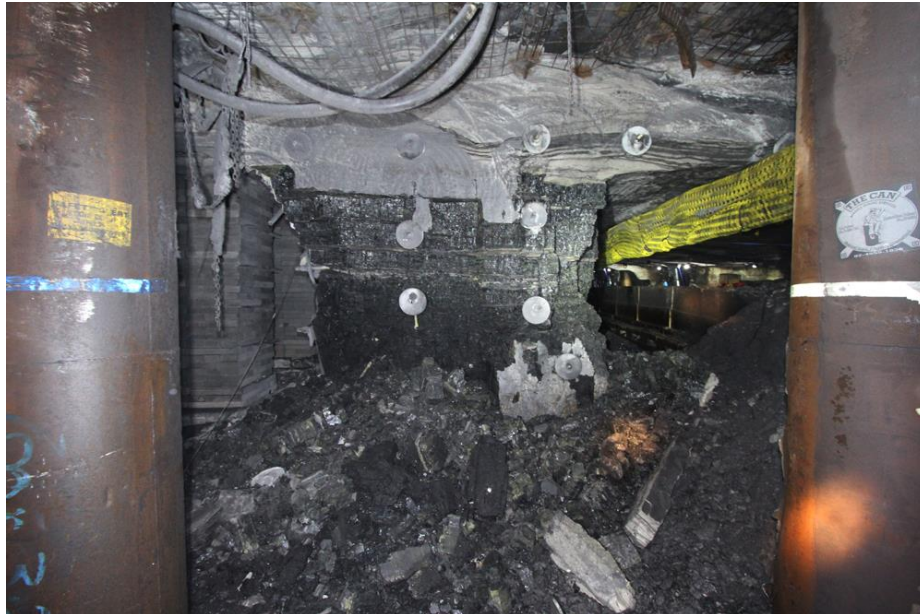
Figure 5: Longwall 20 fender 2.5 m thick
